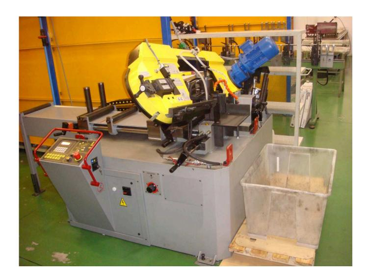
Seeing the importance of the weights in the decorative articles, and having these the need for metallic insertions, DECOREX bets and invests in machinery of automatic cut for metals.
